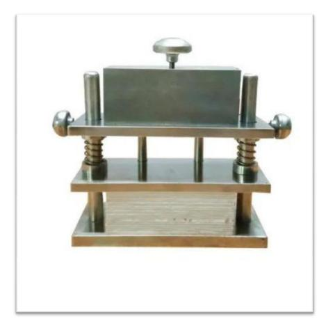
Perspiration is usually liable for the change in color of the material. It's testing equipment which is employed to work out color fastness of dyed or printed fabric against perspiration thanks to water, sea water etc. and sublimations during storage. It's carried on by exposing the material sample to the action of the both acidic and alkaline medium during a controlled temperature and pressure alongside an undyed sample.
