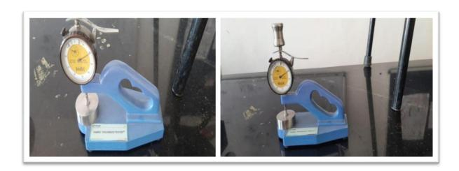
The fabric thickness is usually measured as the distance between the two fabric surfaces under a certain level of applied pressure, depending on whether nonwovens are high loft.
